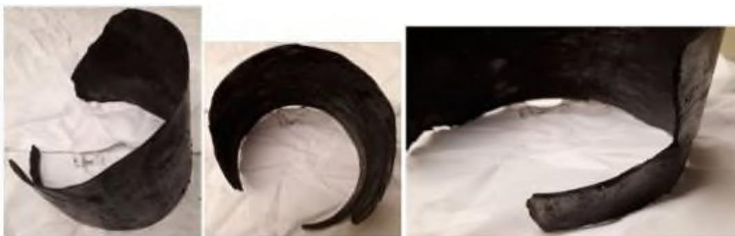
*Image 4: Metals spray coating that was under the 1<sup>st</sup> Intermediate shaft gear. This failed initially at the metal spray coating at the keyway.*
