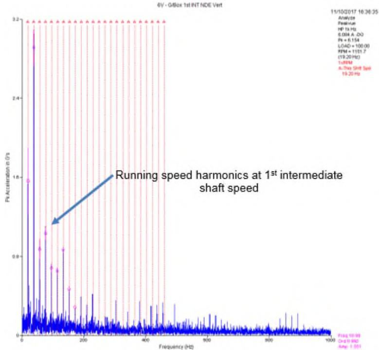
Figure 3: Velocity spectrum taken from the non-drive end (NDE) of the 1st intermediate shaft.
