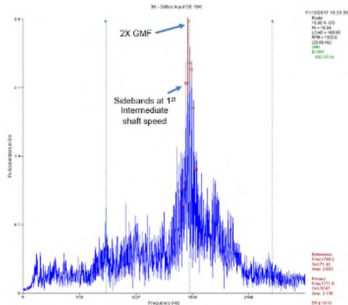
Figure 1: The input shaft high frequency Acceleration spectrum.
