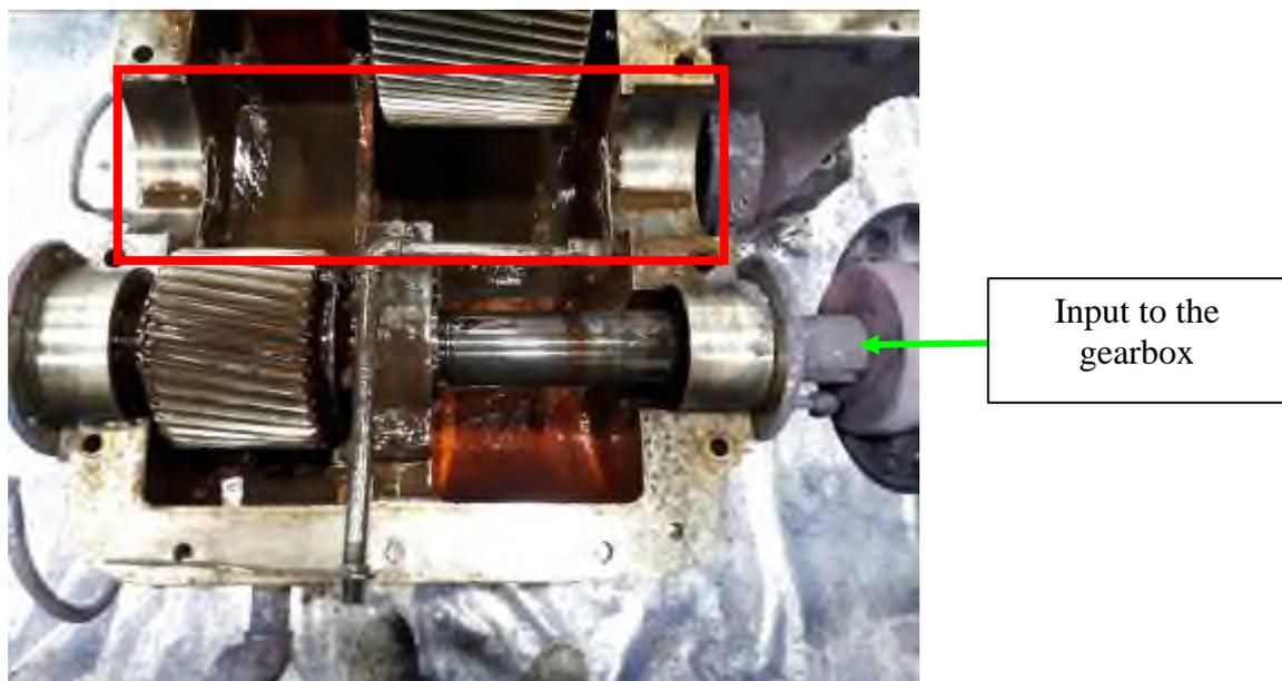
*Image 2: A close view up of the problem shaft location after removal for repair.*
