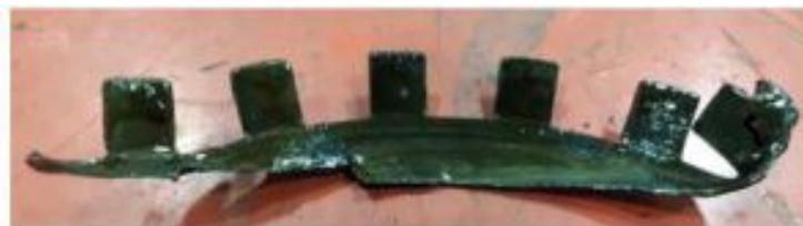
*Image 3 of the failed tab washer found in the bearing cap from the 1<sup>st</sup> Intermediate shaft.*
