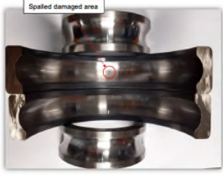
Image 1 is the drive end bearing sectioned and cleaned.
